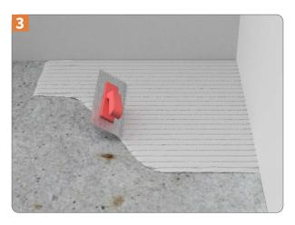
Ultralight should be installed using a flexible, cement-based adhesive. The adhesive should be trowelled out and combed through using a 6 mm x 6 mm ( $\frac{1}{4}$ " x  $\frac{1}{4}$ ") square notch trowel to give a ribbed bed, any slight depressions in the subfloor being filled by the mortar.
